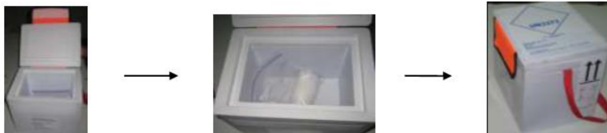
Figure 5: Left: an open safety box; Middle: after inserting the sputum container; Right: after sealing the box.
